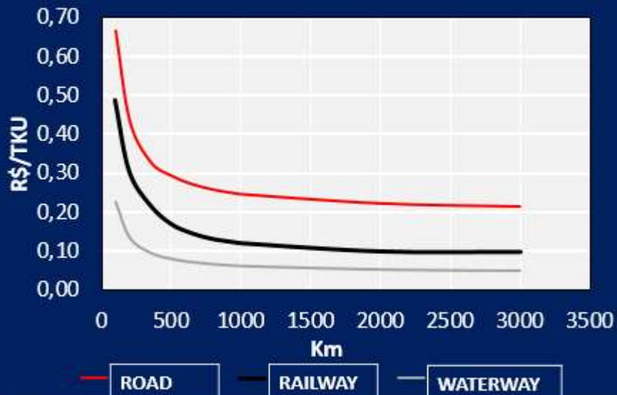
BRAZIL TRANSPORTATION COSTS RELATED TO A 1000 KM TRIP TO THE AGRICULTURAL BULK SOLID CATEGORY
